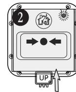
Push upwards - the LED must light on /
