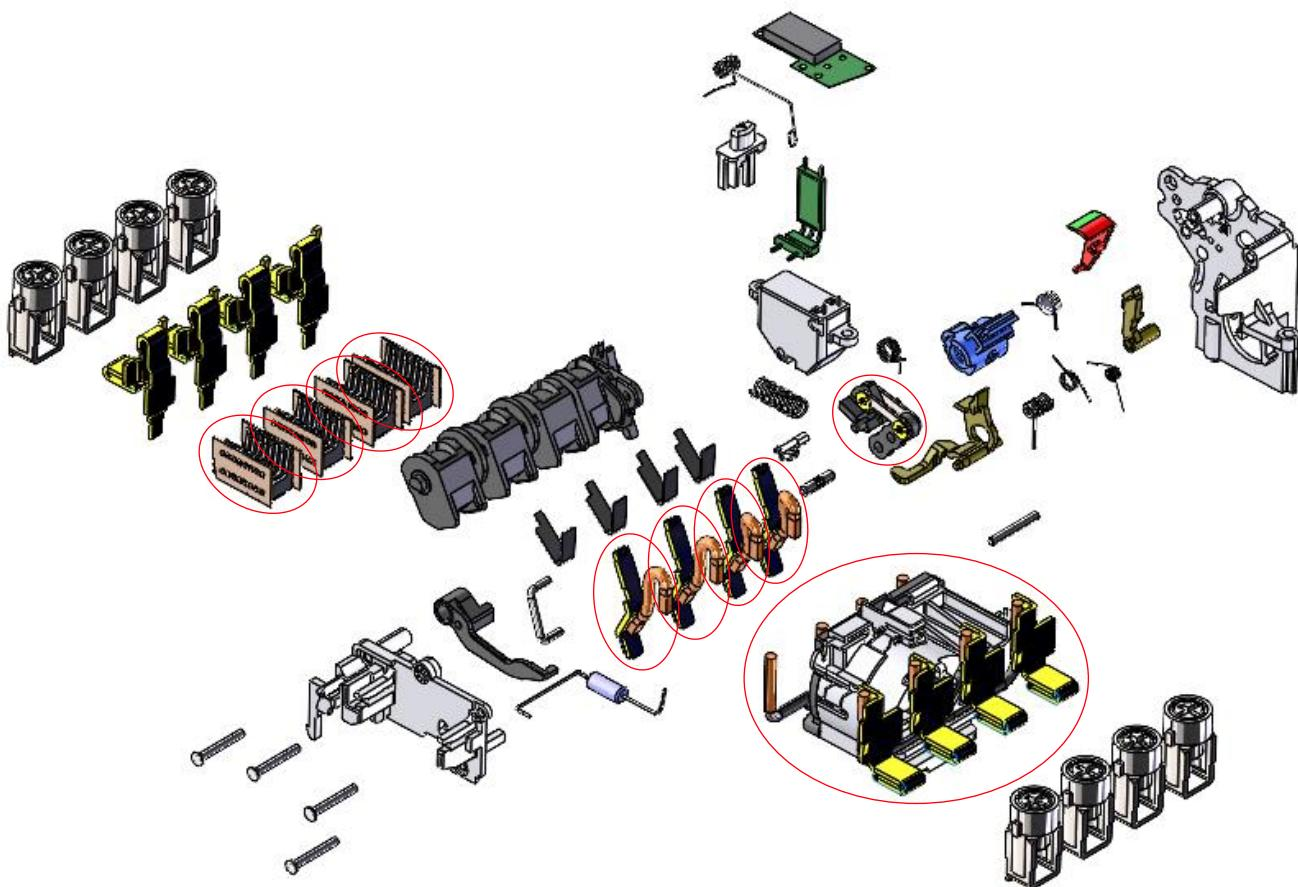
\*Rounded parts have soldered or riveted pieces that cannot be manually disassembled.
