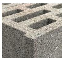
Hollow blocks made from lightweight concrete
