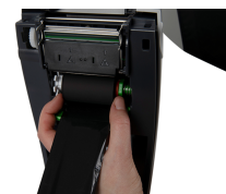
Insert the entire core of the ink ribbon at the bottom.
