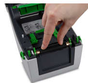
Secure the appropriate roller in the printer.
