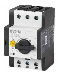
The PKZ-SOL string circuit-breakers are a fuseless alternative for protection against short-circuit currents. Thanks to their variable tripping range, they can be optimally adjusted to the actual short-circuit current of the string. The thermal release will already respond if the current is exceeded by a factor of 1.05 to 1.3, while the magnetic release will trip at six times the current. Open string circuit breakers are designed for installation in customer-specific generator junction boxes.
