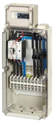
The compact, plug-and-play network and system protection combinations are suitable for systems from 30 kVA to 130 kVA and come in a plastic housing with IP65 protection. Both series meet the requirements of VDE-AR-N 4105:2018-11.
