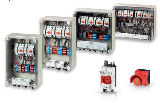
PV fireman's switches are a type of DC switch-disconnector that isolates the cables between the inverter and the solar modules. They enable firefighters to extinguish fires safely.
