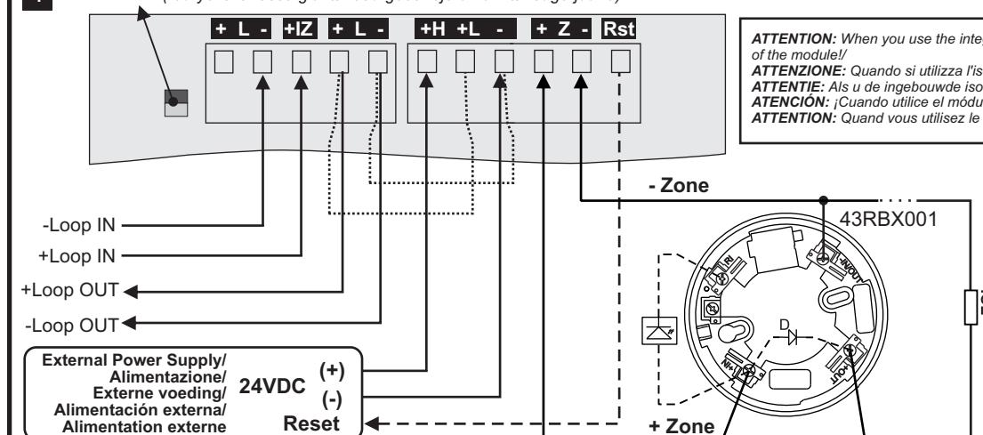
**ATTENTION:** When you use the integrated short circuit isolation module connect one of the "+Loop" loop lead to the "IZ" terminal of the module!
