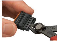
Coding a female connector by removing coding finger(s). (MCS MINI SL)
