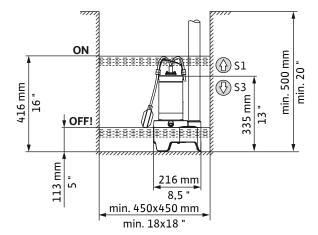
Fig. 2: Installation dimensions and switching points
