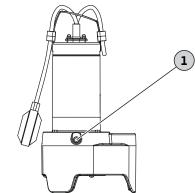
Fig. 3: Sealing chamber oil change
