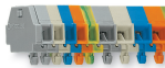
Terminal strip with snap-in mounting feet, for 0.6 ... 1.2 mm plate thickness, 3.5 mm mounting hole diameter (also for 210-154 Aluminum Rail or with 209-120 Mounting Foot for DIN-35 rail)
