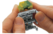
Terminal strip with snap-in mounting feet Snapping a mounting foot (209-120). (Distance between mounting feet: approx. 25 ... 30 mm)
