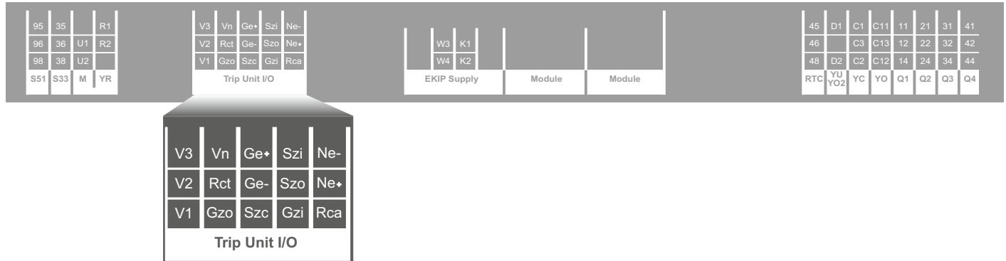
24) RC residual current sensor input (ANSI 64&50N TD) 24a) RC differential ground fault protection sensor input (ANSI 87N)
