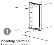
Mounting screw x 4 Screw shaft: Ø4 mm Screw length: ≥ 25 mm
