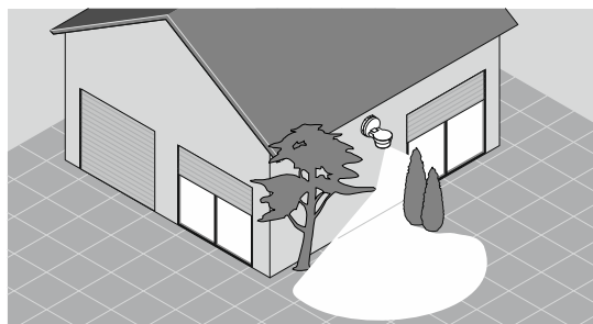
Fig. 20: Wall mounting on free-standing one-family house with limited detection range
