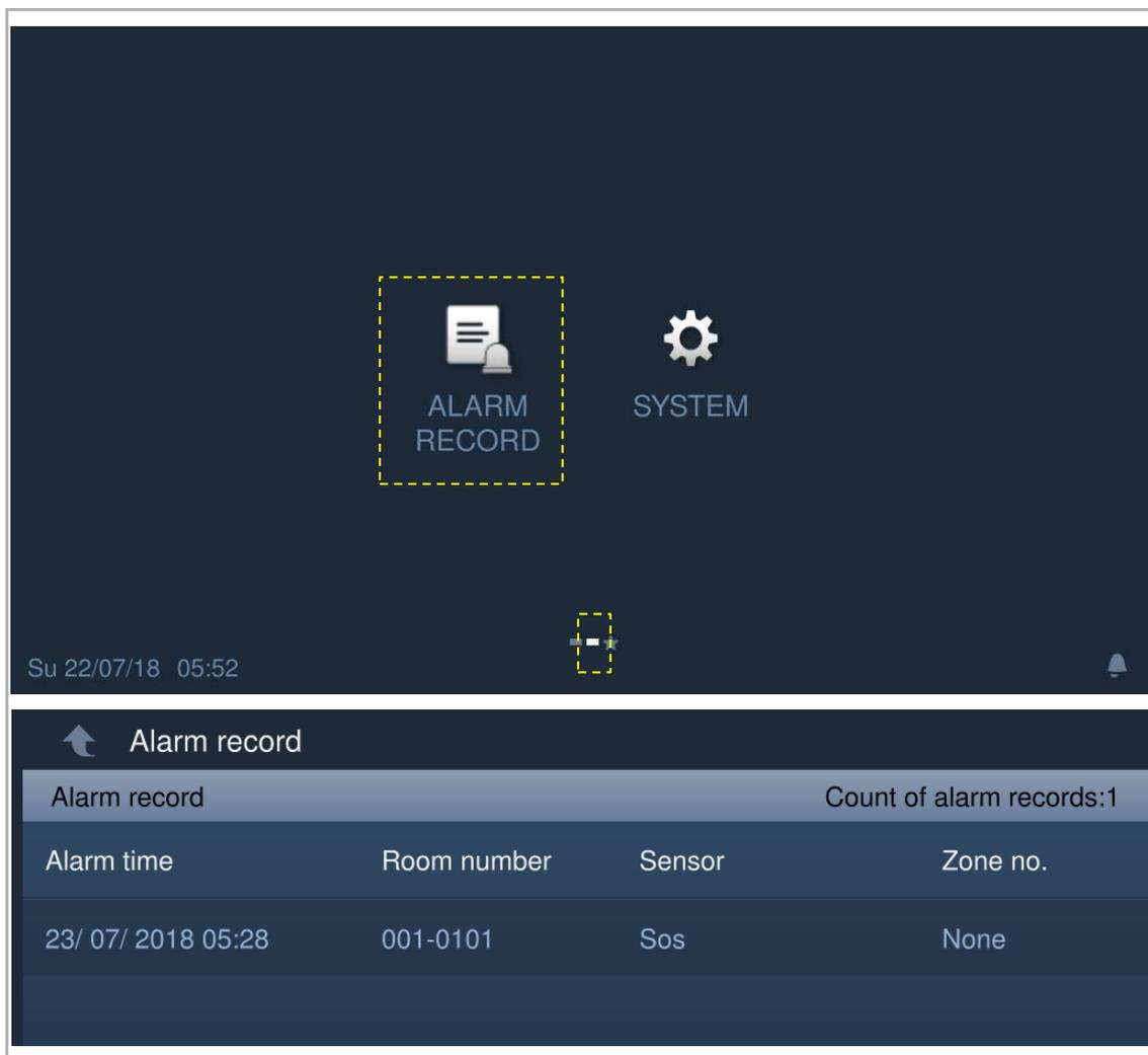
The guard unit will display the alarm message and paly the alarm sound if there is an alarm (e.g. SOS, zone alarm, duress alarm, tamper alarm) is sent from the indoor station or the outdoor station.
