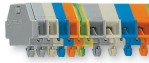
Terminal strip with snap-in mounting feet, for 0.6 ... 1.2 mm plate thickness, 3.5 mm mounting hole diameter (also for 210-154 Aluminum Rail or with 209-120 Mounting Foot for DIN-35 rail)
