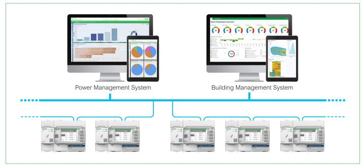
Supports https, SNTP, DHCP, Modbus TCP/IP, BACnet/IP protocols.
