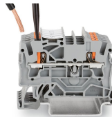
Insert fine-stranded conductors via operating tool.
