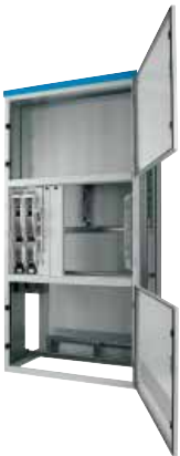
Outgoing section for fuse strips up to 630A alternatively with dropper busbar up to 800-3200 A across two sections
