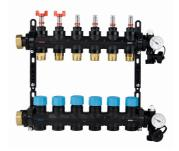
**Commercial information** Composite manifold for both housing and utility buildings. It is compact in construction and has adaptable fixing brackets, it therefore allows smooth installation. This manifold is equipped with flowmeters, control valves for each circuit. Outlets are connected to eurocone 3/4".
