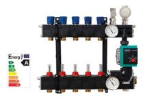
Commercial information Composite manifold for both housing and utility buildings. It is solid in construction and allows smooth installation. The double hollow rooms in the body gives it excellent insulation capacities. This manifold is equipped with flowmeters, control valves for each circuit and water coming from the boiler is reduced to a temperature suitable for underfloor heating. Outlets are connected to eurocone 3/4".
