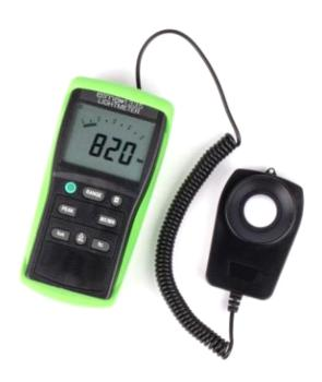
Elma 1335 is a new versatile luxmeter for proper measurement of many types of light. The instrument has a very wide measuring range from 0 to 400,000 lux, which makes it suitable both for emergency lighting and outdoor measurement in strong sunshine. Elma 1335's large display with bargraph and peak, min, maxhold, relative measurement, and zeroadjustment.. The instrument is supplied with bag and external sensor.
