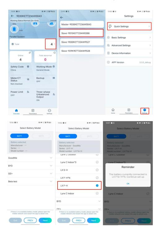
• When setting the parameters of the parallel system, please make sure that the working mode of each inverter is consistent.
