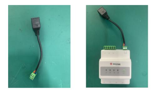
Plug the network cables from the accessory pack into the Meter port of the inverter and the port of the GM330 adapter.
