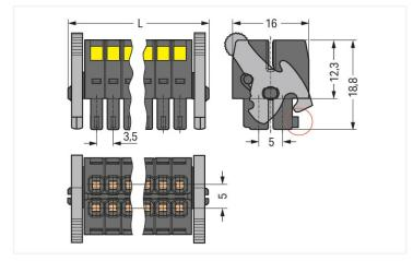
Dimensions in mm L = [(pole no./2) - 1] x pin spacing + 12.2 mm Coding finger (red circle)
