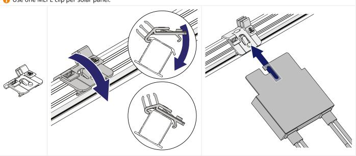
1 With vertical rail orientation you have to fix the MLPE clip by bending the edge of the mounting rail with adjustable pliers.
