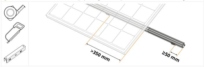
b. If the calculated overhang is less than 250mm beyond the marked position of the last seam clamp, keep 20-35mm rail length overhang for mounting the end cap (art. no. ) (>40mm for the ClickFit EVO 60mm clamp).
