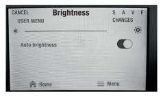
There is a BACK button at the top left of each menu window to enable you to go back one step in the operating process. If something is changed in a window, the Save button appears at the top right.
