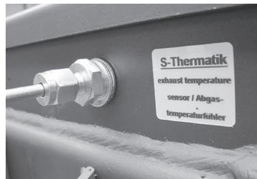
The connection line is routed to the control system where it is connected to the corresponding connection terminal. Pay attention to polarity.
