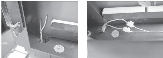
To replace the door switch, unscrew it and pull it upwards. Then unfasten or cut through the cables. Connect the new door switch to the existing wires using individual luster terminals.
