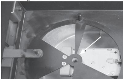
9. Disconnect the cable connector to the actuator motor. With stoves, disconnect directly at the motor. With fireplace inserts, disconnect at the cable connector.
