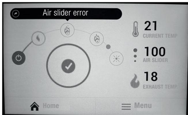
It is NOT permitted to start up the fireplace while an error is active. Contact your stove fitter to inspect the system.
