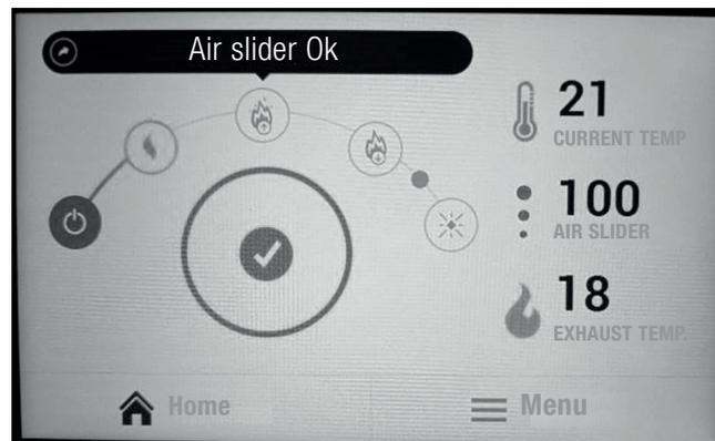
Note: For technical reasons, the air slider test can only be performed with motors of type I (servo motor), but not with motors of type II (spring return). If an obstacle blocks the travel path of the damper slat, the damper slat will become deformed. A sufficiently large air cross section remains.
