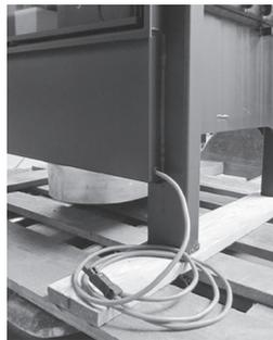
With fireplace inserts, the door contact protrudes from the carcass. It is connected directly to the S-Thermatik NEO. On stoves, the door contact is already connected.
