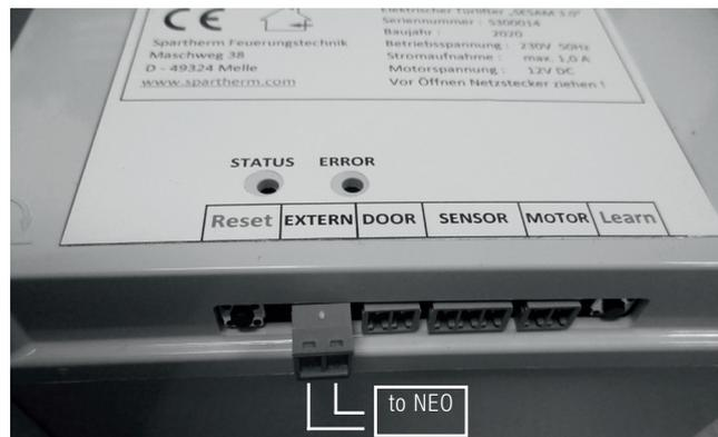
The polarity of the cores is irrelevant.
