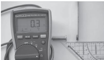
To check the magnetic door contacts, connect them up to an ohmmeter and move a magnet up close to them. The resistance when interconnected should not exceed max. 2.00 Ohms.
