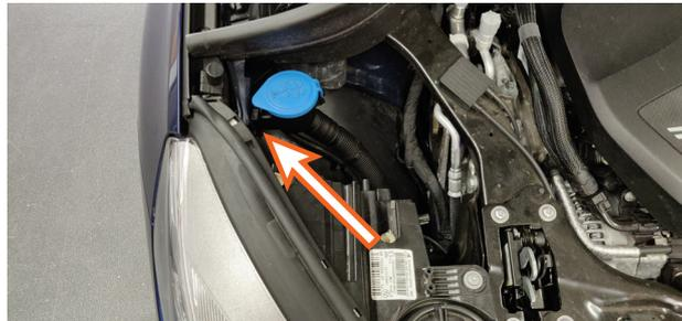
F45/46: Remount the windshield washer fluid reservoir.<sup>5)</sup>
