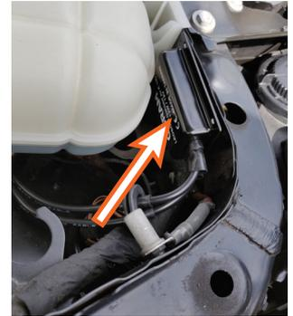
Mount the SMART CANBUS (load resistor) to the vehicle's body (metal).
