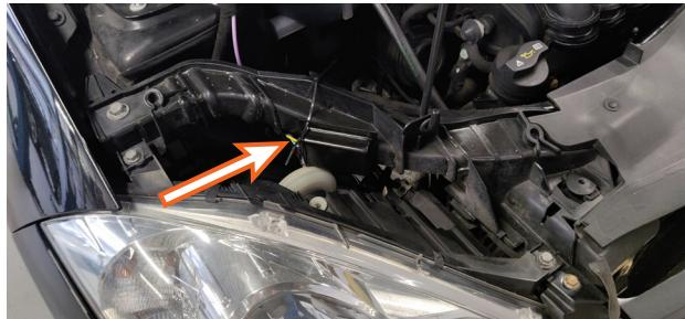
**Mount the SMART CANBUS (load resistor) to the vehicle's body (metal).**
