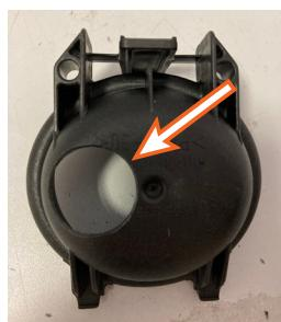
**Mark the headlight protective cover where the hole needs to be drilled.
