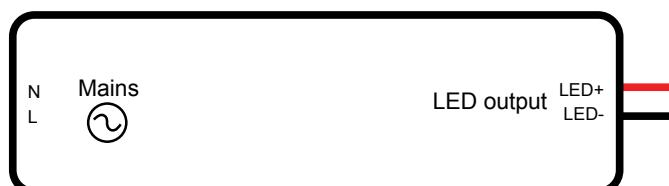
If applicable, connect the Phase dimmer in series on the L-line.
