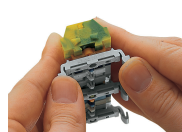
Terminal strip with snap-in mounting feet Snapping a mounting foot (209-120). (Distance between mounting feet: approx. 25 ... 30 mm)
