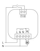
Install JAL-01 in the appliance box behind a push button or in a junction box close to the motor.
