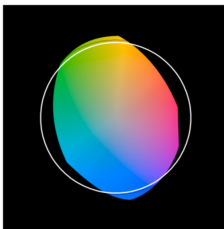
TM30 Colour distortion
