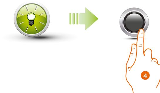
4. Press and quickly release the programming pushbutton, or wait 30 seconds to exit the programming procedure.
