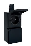
gland. Each socket outlet has an integral closure and is hermetically sealed onto the double box. The fixation points of this double, vertical box are situated 120 mm apart on a vertical axis. This size indication is indelibly imprinted on the bottom of each box. The oval screw openings allow for imprecise drilling. By forming a pressure lock, a gasket ensures the protection degree and the double insulation. The box contains two diagonal, knock-out condensation openings.
