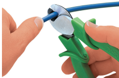
Cutting a cable.
