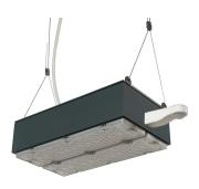
Logistics and Industry high bay luminaire with wide optics to provide homogenous light distribution for open space areas. 9300lumens, 54W, 172lm/W, 4000K, CRI80, wide beam optic. Fitted with a high bay PIR for 360° detection up to 16m range at 15m mounting height.3 step MacAdam ellipse, grey finish (RAL7012), Class 1, 220-240V, IP65, IK06 (sensor IK03).
