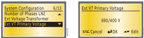
Figure 7.15 Ext VT Primary Voltage, factory setting is 690/400V
