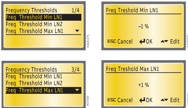
Figure 7.36 Frequency Threshold LN1, factory settings: min -1%, max 1%
