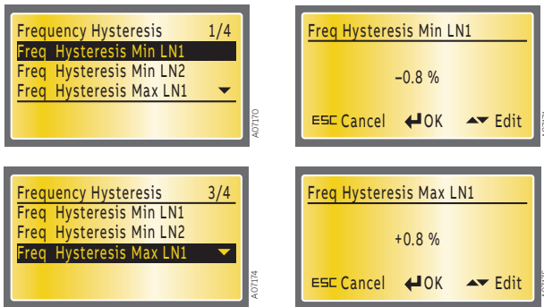
Figure 7.38 Frequency Hysteresis LN1, factory settings: min -0.8 %, max 0.8 %
