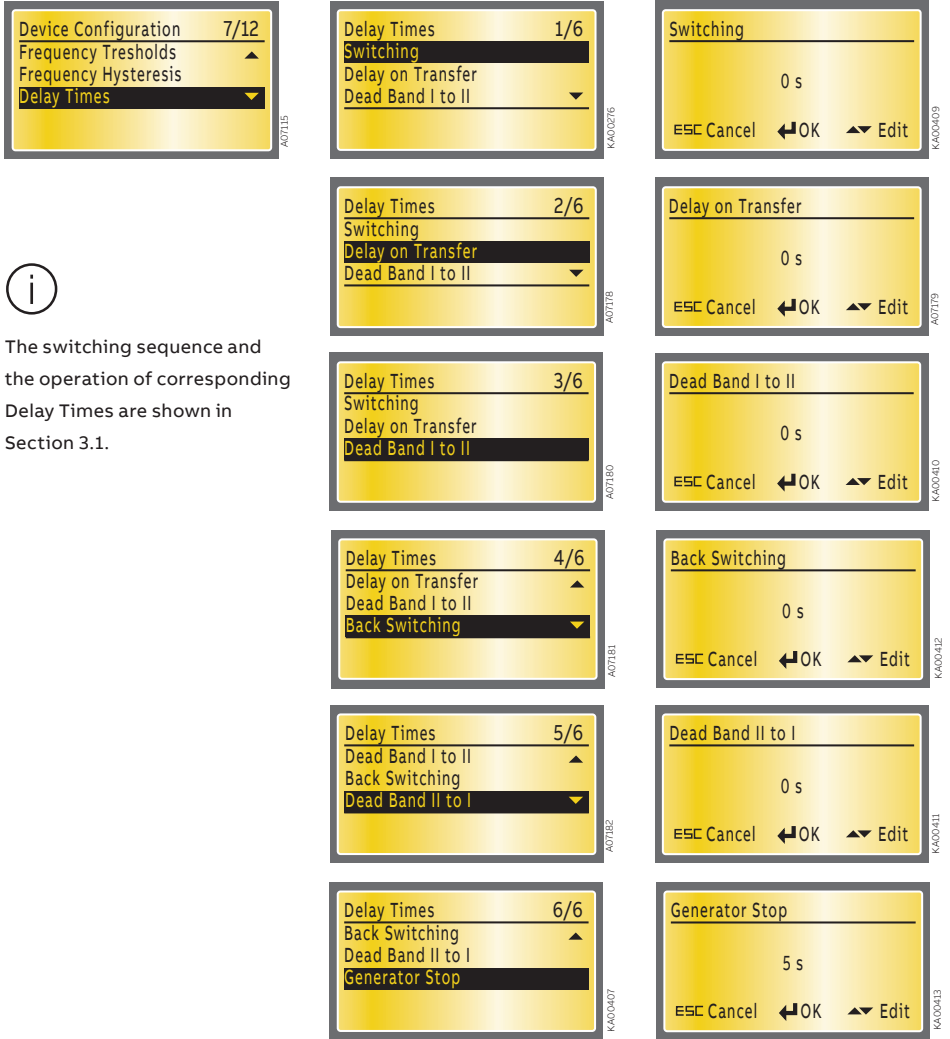
Figure 7.40 Switching 0 s, Delay on Transfer 0 s, Dead Band I to II 0 s, Back Switching 0 s, Dead Band II to I 0 s, Generator Stop 5 s
