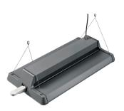
· Logistics and Industry modular high bay luminaire with wide optics to provide homogenous light distribution for open space areas. Twin body with 6 optical modules, 47400 lumens, 327W, 145lm/W, 4000K, CRI 80, wide beam optic. Fitted with a high bay PIR for 360° detection up to 16m range at 15m mounting height. 3 step MacAdam ellipse, grey finish (RAL7012), Class 1, 220-240V, IP65, IK08 (sensor IK03), (LxWxH) 726x386x133mm, Mains + control cable of 2 meter.
