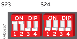
Figure 7.6 DIP switches in OMD200 and OMD300, the positions are factory default settings
