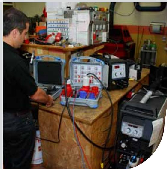
The A 1422 Multifunctional test adapter has all functionalities as its predecessor A 1322 plus complete support for testing of Arc Welding Equipment. This makes it a perfect test and troubleshooting instrument for the demanding user.
