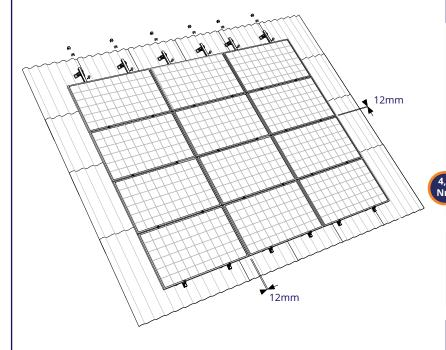
1 MOUNT THE TOP SOLAR PANEL ONTO THE RAILS
