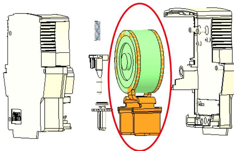
\*Rounded parts have welded pieces that cannot be manually disassembled.
