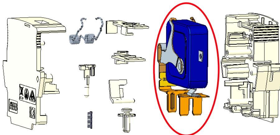
\*Rounded parts have welded pieces that cannot be manually disassembled.
