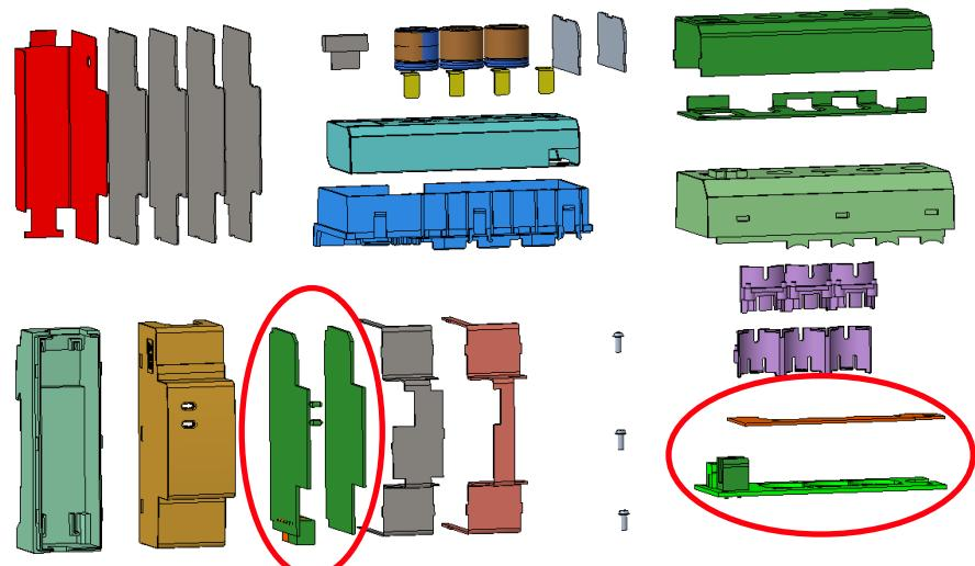
\*Rounded parts have welded pieces that cannot be manually disassembled.
