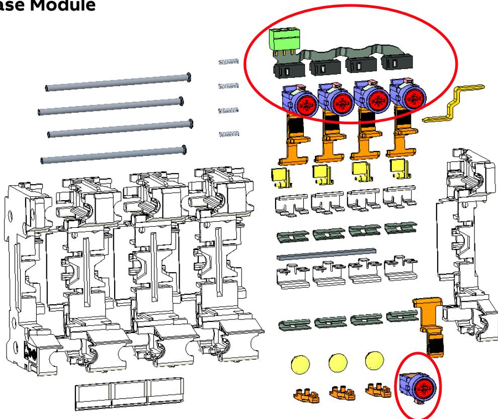
\*Rounded parts have welded pieces that cannot be manually disassembled.
