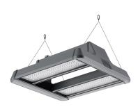
· Logistics and Industry modular high bay luminaire with wide optics to provide homogenous light distribution for open space areas. Single body with 2 optical modules, 14200 lumens, 95W, 150lm/W, 4000K, CRI 80, wide beam optic, DALI dimmable, 3 step MacAdam ellipse, grey finish (RAL7012), Class 1, 220-240V, IP65, IK08, (LxWxH) 410x386x133mm, Mains + control cable of 2 meter. Ball-impactresistance according to VDE 0710-13 in suspended mounting mode.
