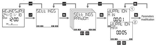
The "random switching O" function (activated with the combination described on page 6) allows the channel on which it's active to automatically switch and at random time intervals.
