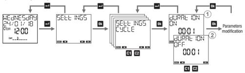
The "cycle switching" function (activated with the combination described on page 6) is a succession of on and off switching. The cycle programme always starts from the on status. In this menu it's possible to define the duration of on and off. The duration of the on and off duration cannot be less than one minute. Default on duration: I minute, OFF duration: I minute
