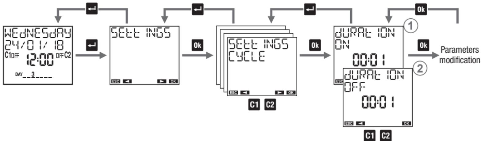
The “cycle switching” function (activated with the combination described on page 6) is a succession of on and off switching. The cycle programme always starts from the on status. In this menu it’s possible to define the duration of on and off. The duration of the on and off duration cannot be less than one minute. Default on duration: 1minute, OFF duration: 1 minute
