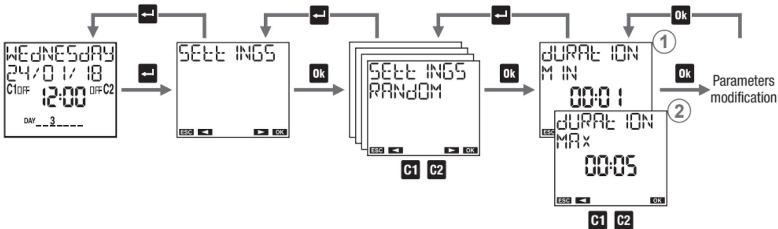
The “random switching ②” function (activated with the combination described on page 6) allows the channel on which it’s active to automatically switch and at random time intervals.
