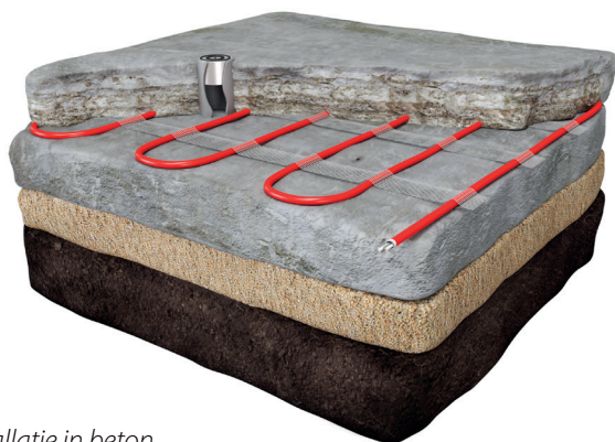
Installatie in beton
