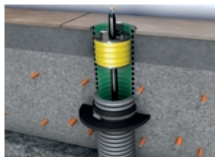
Application: Waterproof concrete wear class 1 and 2 W1-E according to DIN 18533
