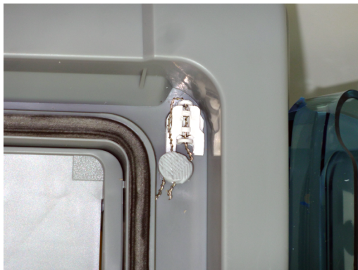
Sealing the screws on the front panel.
