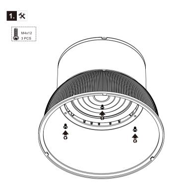
Install the Anti-glare diffuser body to LED high bay with 3 supplied screws.
